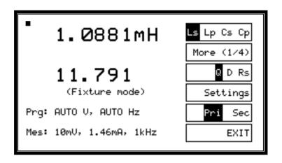
The ATi is making measurements on nodes 13 and 15 (the 'primary') and nodes 14 and 16 (the 'secondary'). The LCR fixture supplied with your ATi has four Kelvin leads already connected to these nodes.
