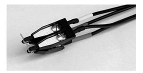
To perform open-circuit compensation for stray capacitance, remove all parts under test but leave the BNC leads or test fixture in place and press softkey 2 'Open' and select '**One'** or '**All**'.For optimum accuracy, place any leads or other connectors that can move in a position as close as possible to that which will be used when making measurements.
